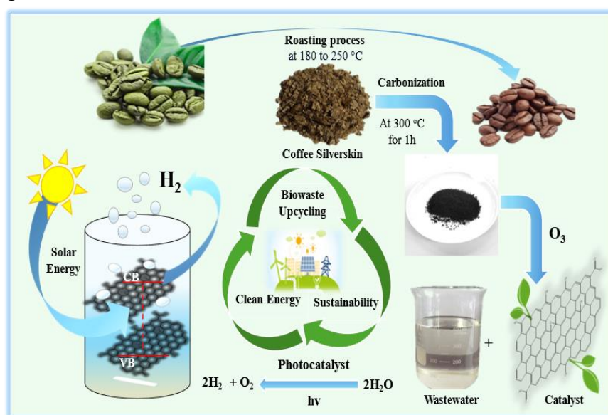
Figure 1. SGO production process and its application for solar driven promoted H 2 production
