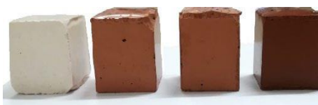
Figure 1. Red mud-metakaolin based geopolymers cubes.
